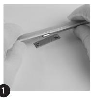
Fix optional steel plates (if using) with suitable countersunk screws (min. 4 steel plates per metre/40").
